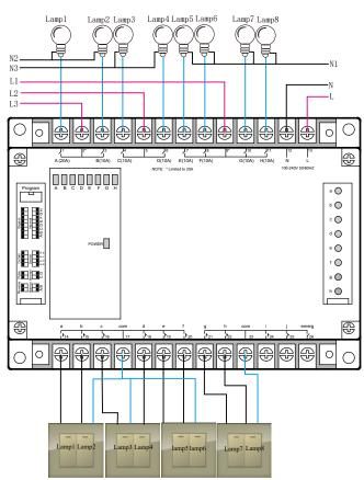
B: Being configurated as 3-Ch. curtain + 2-Ch. relay outputs
